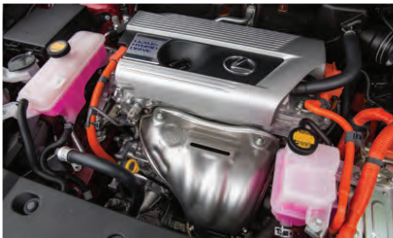
For safety's sake, high-voltage cables are COLOR-CODED ORANGE .
