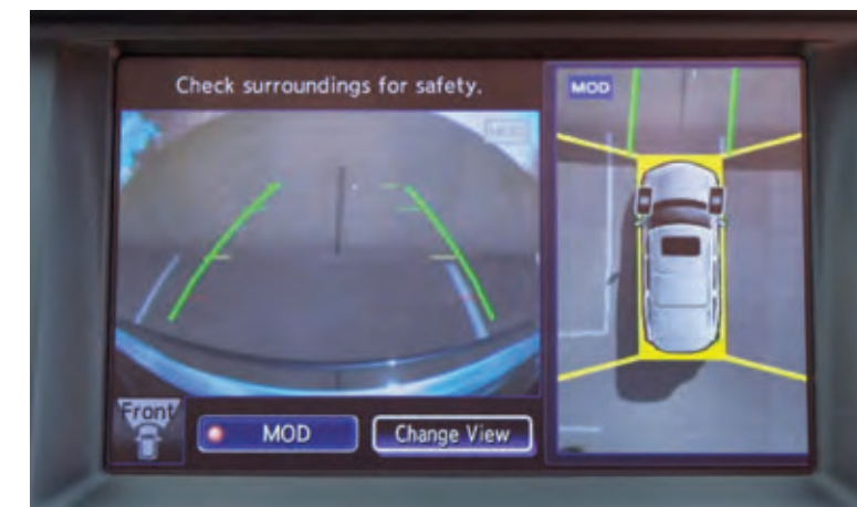
Rearview cameras are yesterday's news. The latest lenses gives a BIRD'S-EYE VIEW , as depicted in Infiniti's Around View Monitor.
