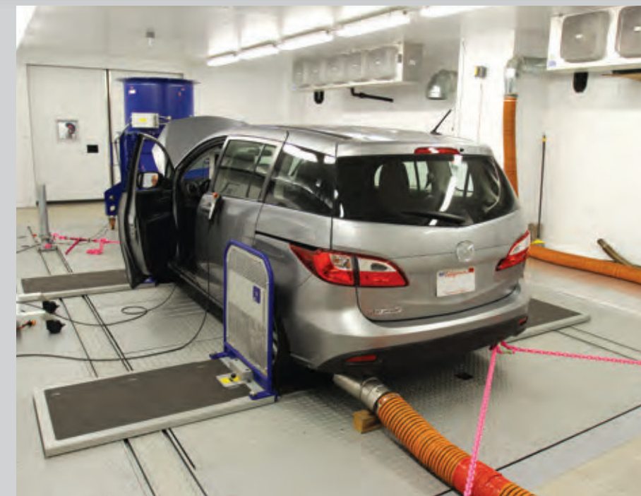
A Mazda5 on the DYNAMOMETER at the Automobile Club of Southern California's Automotive Research Center.
