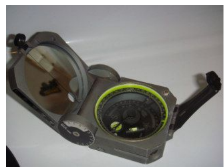
A standard Brunton Pocket Transit, used commonly by geologists in mapping and surveying
