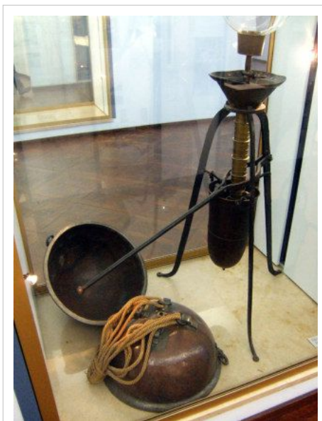
The original Magdeburg hemispheres (lower left) used to demonstrate Otto von Guericke's vacuum pump (right)
