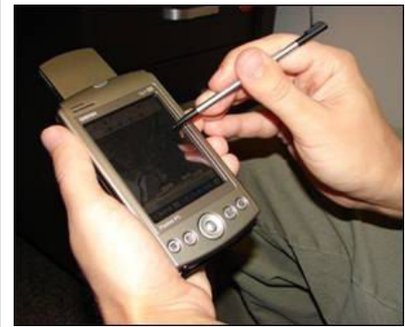
Today, handheld computers with GPS and geographic information systems software are often used in geological field work (digital geologic mapping).
