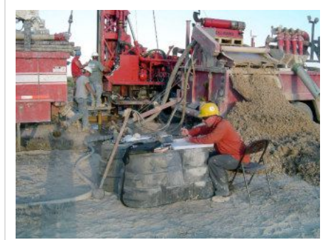
Mud log in process, a common way to study the lithology when drilling oil wells.
