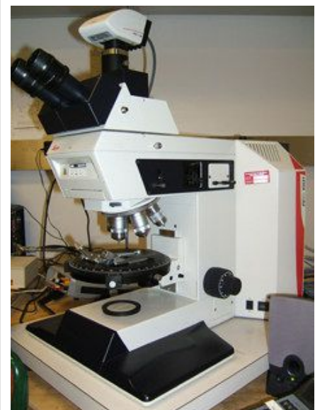
A petrographic microscope, which is an optical microscope fitted with cross-polarizing lenses, a conoscopic lens, and compensators (plates of anisotropic materials; gypsum plates and quartz wedges are common), for crystallographic analysis.
