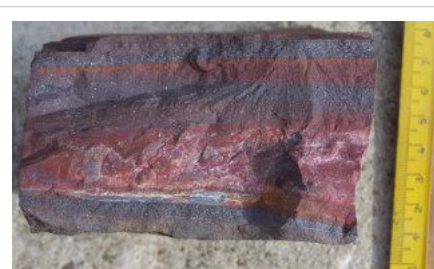
A banded iron formation from the 3.15 Ga Moories Group, Barberton Greenstone Belt, South Africa. Red layers represent the times when oxygen was available, gray layers were formed in anoxic circumstances.
