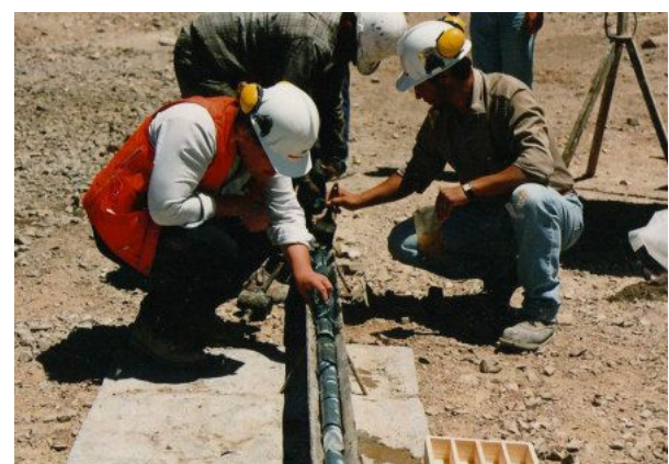
Exploration geologists examining a freshly recovered drill core.
