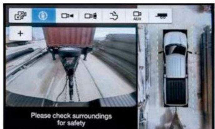
The latest cameras provide drivers with views all around a vehicle, as with the Ford F-150's MULTIPLE-CAMERA DISPLAY .
