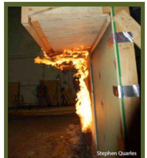
Lateral flame spread was reduced when a combustible soffit material ignited in this test of a soffited-eave with a combustible soffit material.
